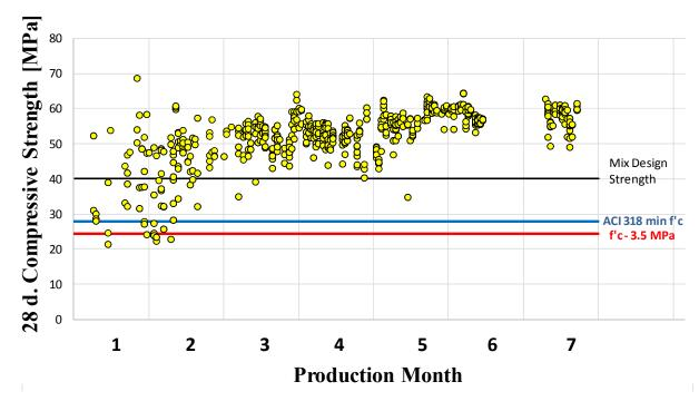
Fig. 3 - 28-day Compressive Strength of 1129 concrete samples
