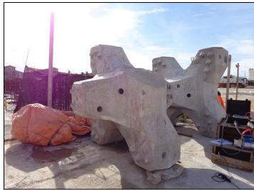
Fig. 4 - Preselected Accropodes<sup>TM</sup> II (broken element at the foreground) ready for testing
