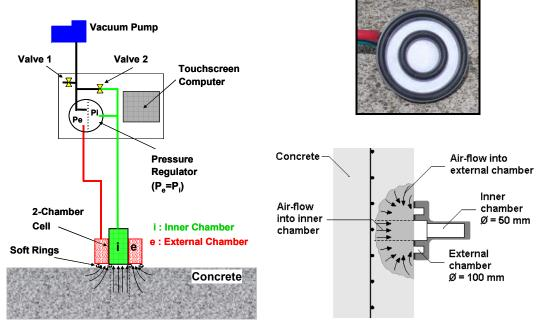
Fig. 7 – Sketch of air-permeability Fig. 8 – Vacuum cell and air-flow into both test. chambers.
